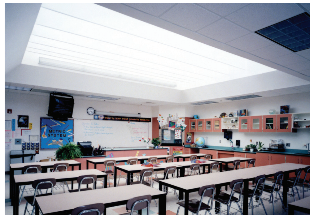
Light colored walls, ceiling and floors improve daylighting performance.
